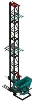
Tiltable Concrete Bucket (0.3 cubic mtr)(Optional)
