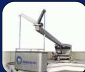
Building Maintenance Unit
